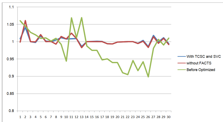
Fig. 10. Voltage profile improvement after allocating the dual device.
